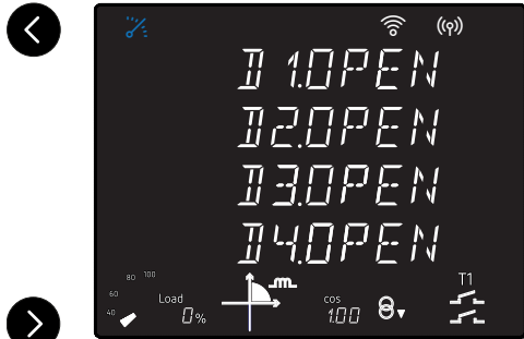
Digital Input 1 status Digital Input 2 status Digital Input 3 status Digital Input 4 status
